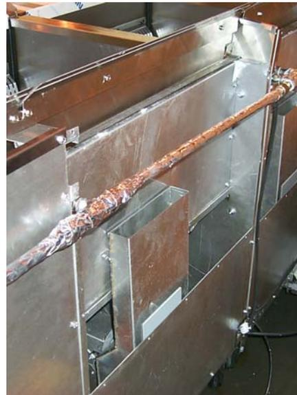
Multi-battered systems after 02/03 have upper and lower back panels, which must be removed to access the blower assembly (fryer above shown with upper back panel removed).
