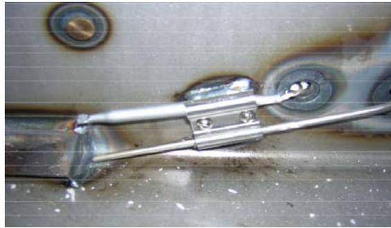
9. On the sensor bulb being removed, loosen and unscrew completely the compression nut, then the pass-through nut from the frypot. Carefully remove the sensor bulb from the frypot, being careful not to damage the remaining sensor bulb.
