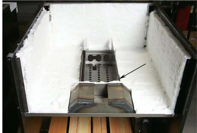
Install new insulation in firebox using spray adhesive, ensuring good contact between insulation and metal surfaces.
